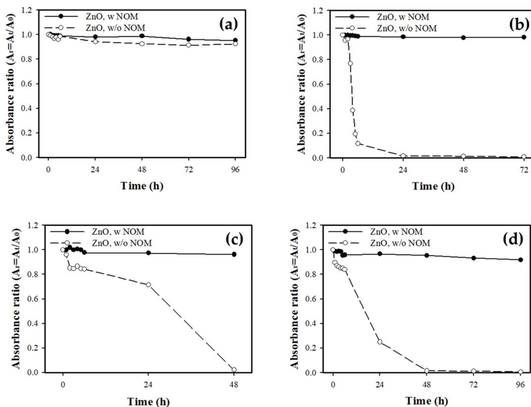
**Figure 1.** Sedimentation kinetics for zinc oxide nanoparticles (ZnO NPs) with/without natural organic matter (NOM) under deionized water (DI) water (a), Organization for Economic Co-operation and Development (OECD) medium (b), International Organization for Standardization (ISO) medium (c), and dechlorinated tap water (d).
