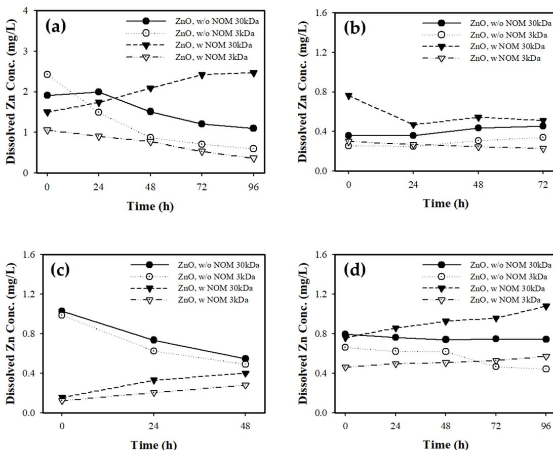
**Figure 6.** Dissolution of ZnO NPs with/without NOM in DI water (a), OECD medium (b), ISO medium (c), and dechlorinated tap water (d).
