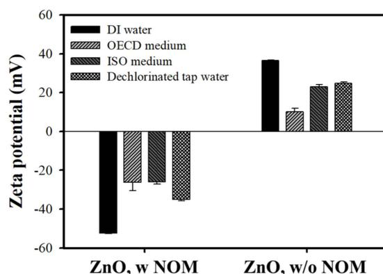
**Figure 3.** Zeta potential of ZnO NPs with/without NOM. Values on the graph represent mean  $\pm$  standard deviation.
