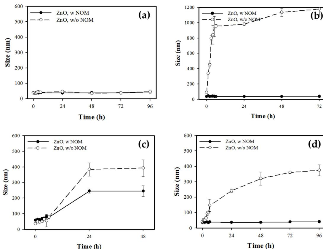
**Figure 5.** Hydrodynamic diameter of ZnO NPs with/without NOM in DI water (a), OECD medium (b), ISO medium (c), and dechlorinated tap water (d).
