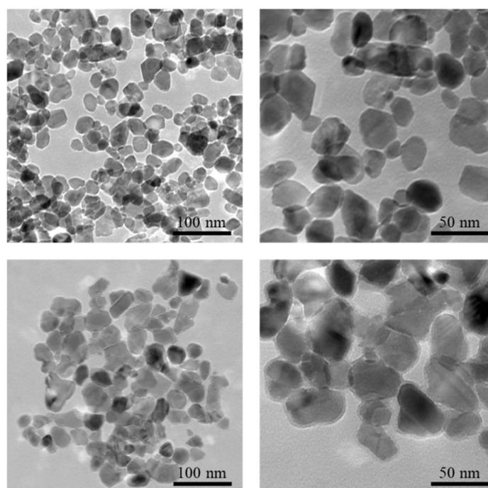
**Figure 2.** Transmission electron microscopy (TEM) image of ZnO. Top (without NOM), down (with NOM).
