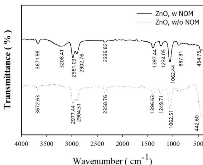
**Figure 4.** Fourier-transform infrared spectra of ZnO NPs with/without NOM.
