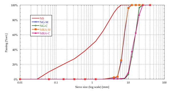
Figure 1. Grading of the aggregates.
