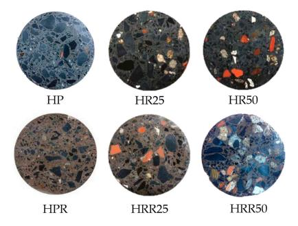
Figure 9. Concrete specimen sections.
