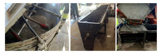
Figure 2. Precast element manufacturing sequence.
