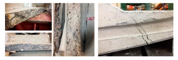
Figure 11. Precast test and cracking.
