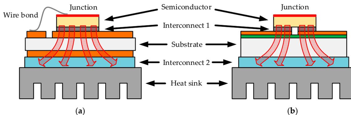
**Figure 1.** Typical thermomechanical set-up for power electronics (a) and solid-state lighting (SSL) (b) in a general manner with heat flow from junction to heat sink through semiconductor, interconnect 1 (single electrical contact in (a) and multi electrical contact in (b)), substrate (direct bonded copper (DBC) in (a) and insulated metal substrate printed circuit board (IMS-PCB) in (b)) and interconnect 2 with a spreading of the heat.
