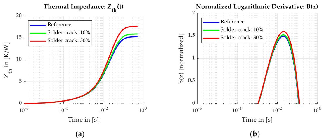
**Figure 4.** Evaluation methods in TTA: (a)  $Z_{th}$  evaluation and (b) normalized logarithmic derivative. Data are generated by an optimized FEM model in a transient thermal simulation with a crack growth of 10% or 30% in the solder joint compared to its area described in [44]. An increase of 0.63 K/W or 2.37 K/W was observed in  $Z_{th}(t)$  and 0.012 or 0.044 in peak increase for  $B(z)$ .
