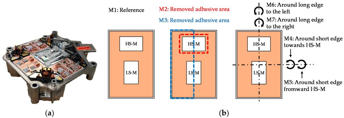
**Figure 9.** (a) Image of the inspected power inverter module in a semi-fabricated state for adhesive investigation with five half bridges on five DBCs attached with nonconductive thermal adhesive to an aluminum body. The sixth DBC holds peripheral components. (b) Schematic description of adhesive manipulations on a single DBC/half bridge used for grouping.
