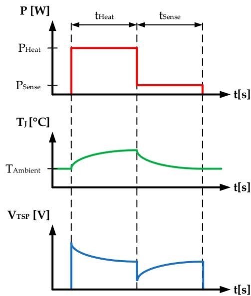
**Figure 3.** Measurement sequence for transient thermal analysis (TTA) with course of power  $P$ , junction temperature  $T_j$ , and voltage of temperature-sensitive parameter  $V_{TSP}$ .
