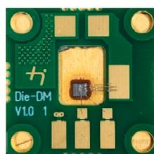
**Figure 7.** Sintered bare die MOSFET on ENIG metallized copper plate with FR4 adapter PCB holding the probing pads for ATIM and Al wire bonds to the MOSFET top contacts.
