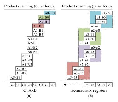
**Figure 2.** The proposed product scanning multiplication. (a) outer loop, an example of 128-bit multiplication. (b) inner loop,  $(A0 \cdot B0, A1 \cdot B0, A0 \cdot B1, A2 \cdot B0)$ .
