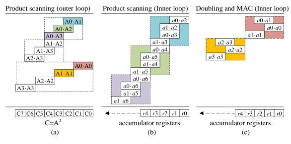
**Figure 3.** The proposed product-scanning squaring. (**a**) outer loop, an example of 128-bit squaring. (**b**) inner loop, product scanning,  $(A0 \cdot A0, A0 \cdot A2, A0 \cdot A3)$ . (**c**) inner loop, doubling and MAC,  $(A0 \cdot A0, A1 \cdot A1)$ .
