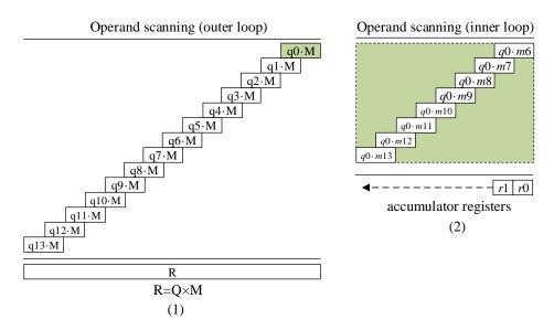
**Figure 4.** Proposed operand scanning multiplication for Montgomery reduction. **Left part**: outer loop, an example of SIKEp434. **Right part**: inner loop,  $(q0 \cdot M)$ .
