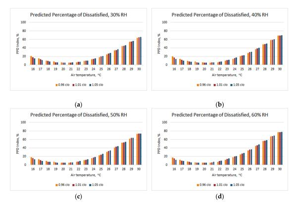
**Figure 5.** PPD index for the surgeon, dressed in three clothing ensembles with different clothing insulation: (**a**) relative humidity (RH) of the air 30%; (**b**) RH 40%; (**c**) RH 50%; (**d**) RH 60%.
