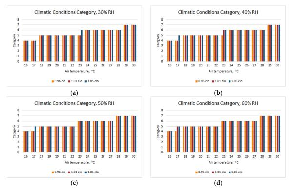
**Figure 6.** Climatic conditions category for the surgeon, dressed in three clothing ensembles with different clothing insulation: (**a**) relative humidity (RH) of the air 30%; (**b**) RH 40%; (**c**) RH 50%; (**d**) RH 60%.
