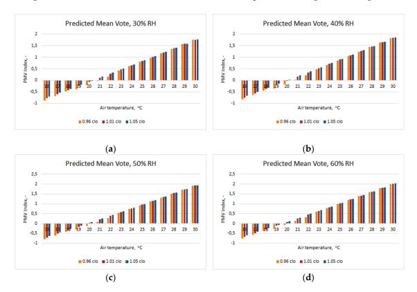
**Figure 4.** PMV index for the surgeon, dressed in three clothing ensembles with different clothing insulation: (**a**) relative humidity (RH) of the air 30%; (**b**) RH 40%; (**c**) RH 50%; (**d**) RH 60%.
