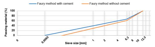
Figure 1. Faury method for reference concrete.
