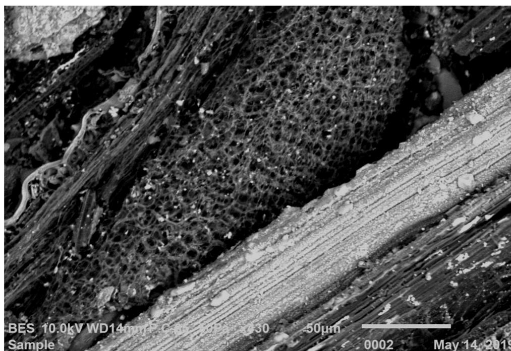
**Figure 2.** Rice straw biochar surface at 1000× magnification under SEM.
