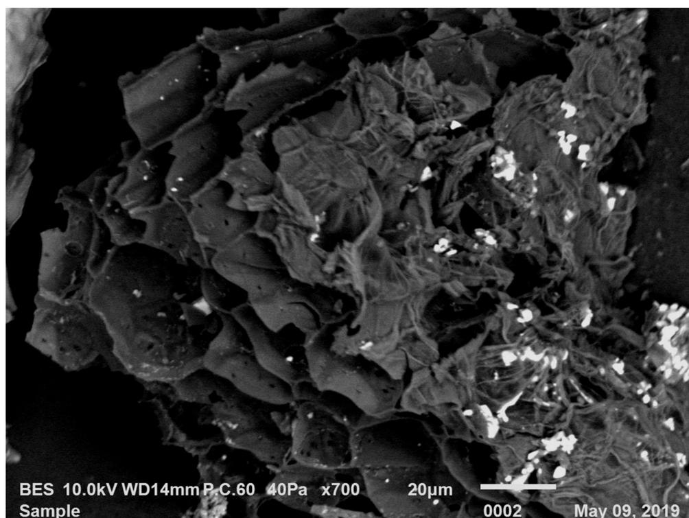
**Figure 1.** Rice husk biochar surface at  $700\times$  magnification under SEM.
