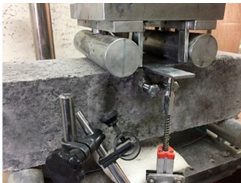
Figure 3. How to adjust the device and sample to test the flexural strength.
