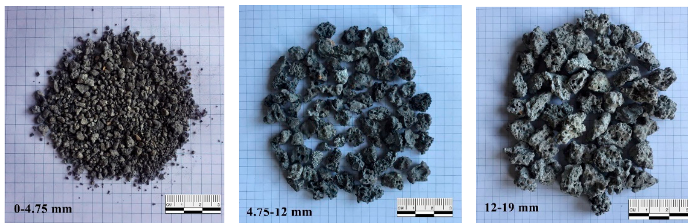
Figure 2. EAFS aggregate sizes used.
