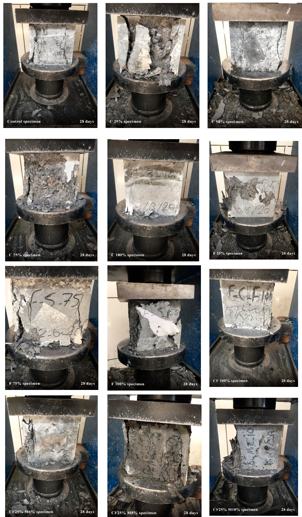
Figure 8. Crack patterns of the different mixes after the compressive strength test.
