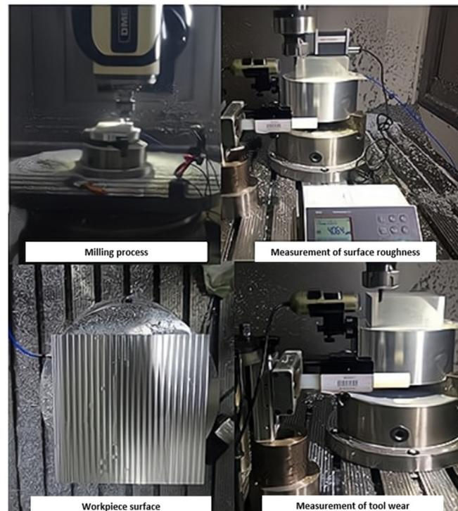
**Figure 7.** Experiment environment and measurement.
