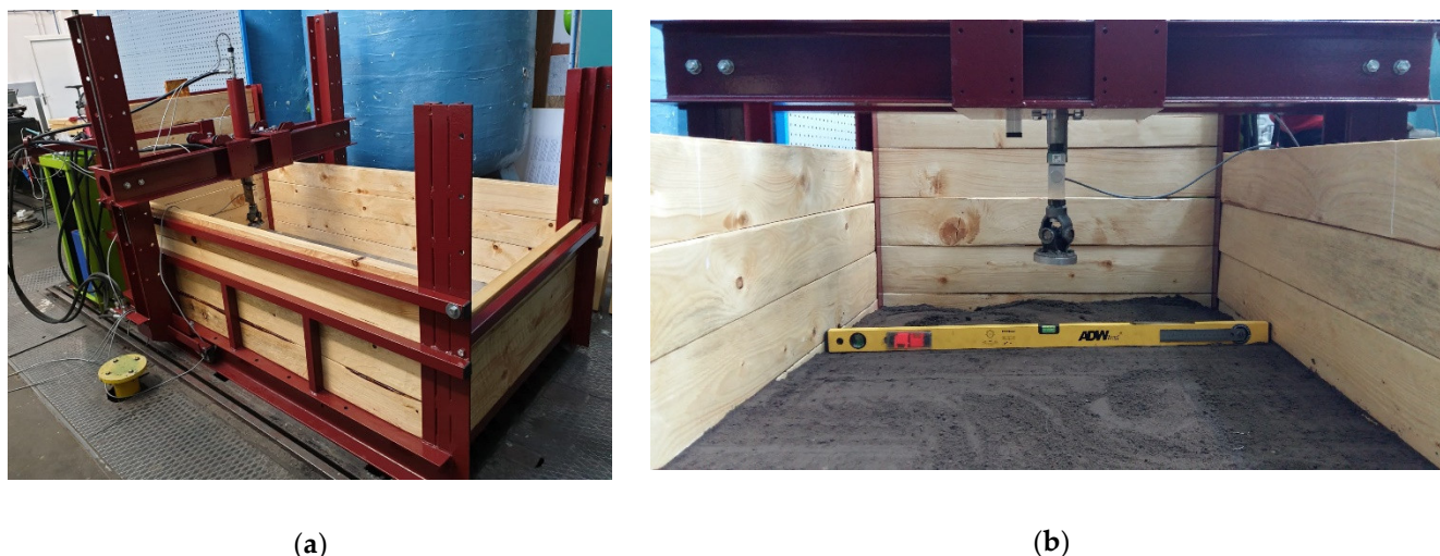
Figure 1. (a) Plate sinkage test (bevameter device); (b) soil surface leveling.
