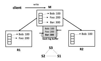
Figure 1. Redis architecture. M, R, and S stand for master, replica, and sentinel, respectively.
