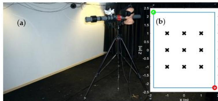
**Figure 2.** Photo of the laboratory room with a tracker and a model of the launcher on a tripod (a); and diagram of the distribution of the measuring points (“x” symbols) (b). The blue line marks the walls of the room, and the red and green circles symbolise the base stations.
