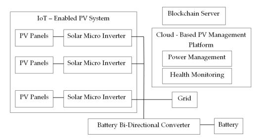
Figure 9. Architecture of IoT-enabled PV system.
