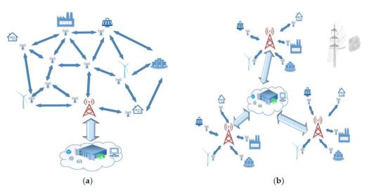
Figure 4. (a,b) shows the schematic of ZigBee (Mesh) and of LoRa (Star).
