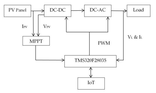
Figure 11. Topology and the control strategy of the IoT-enabled smart inverter.
