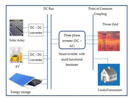
Figure 2. Smart inverter with multi-functional features.
