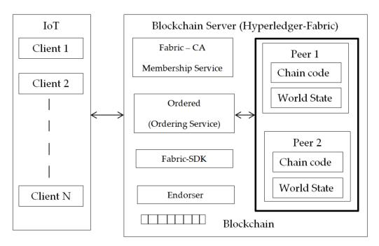
Figure 10. Architecture of blockchain implementation in IoT.
