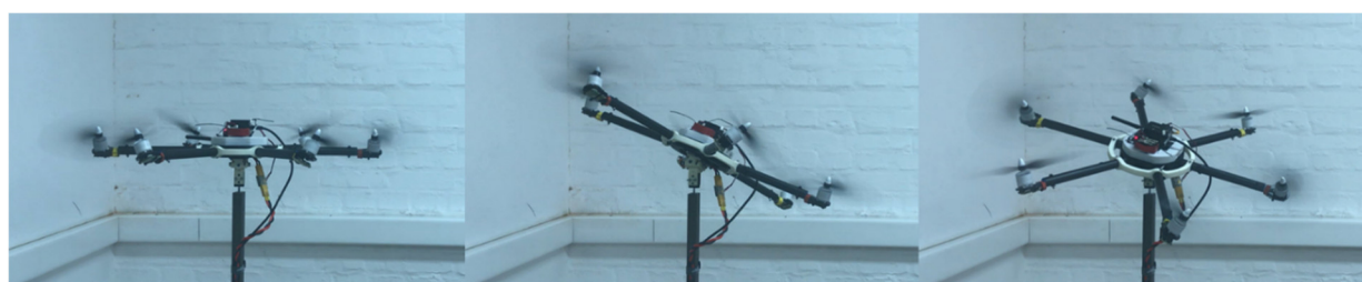
Figure 12. Experimental testing of attitude control on PTX6 for the case of reference state tracking.
