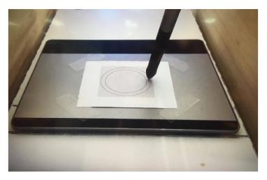
**Figure 3.** The digitizer tablet and modified Endo Babcock clamp with a digital pen used in the circle-tracing task.
