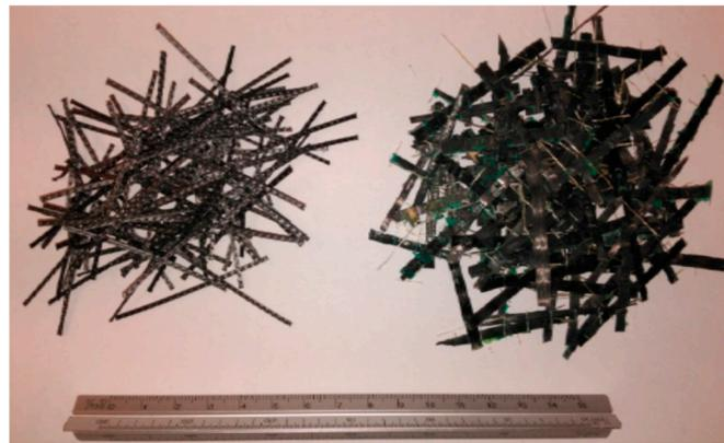
**Figure 1.** Polypropylene fibers and recycled carbon fibers.
