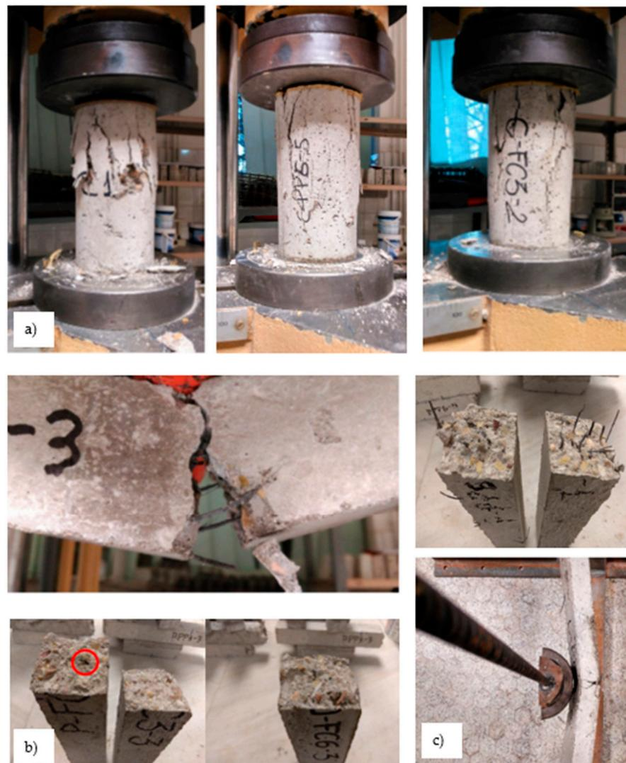
**Figure 8.** Symptomatology of the concrete: (a) compression tests; (b) flexural tests; and (c) impact resistance tests.
