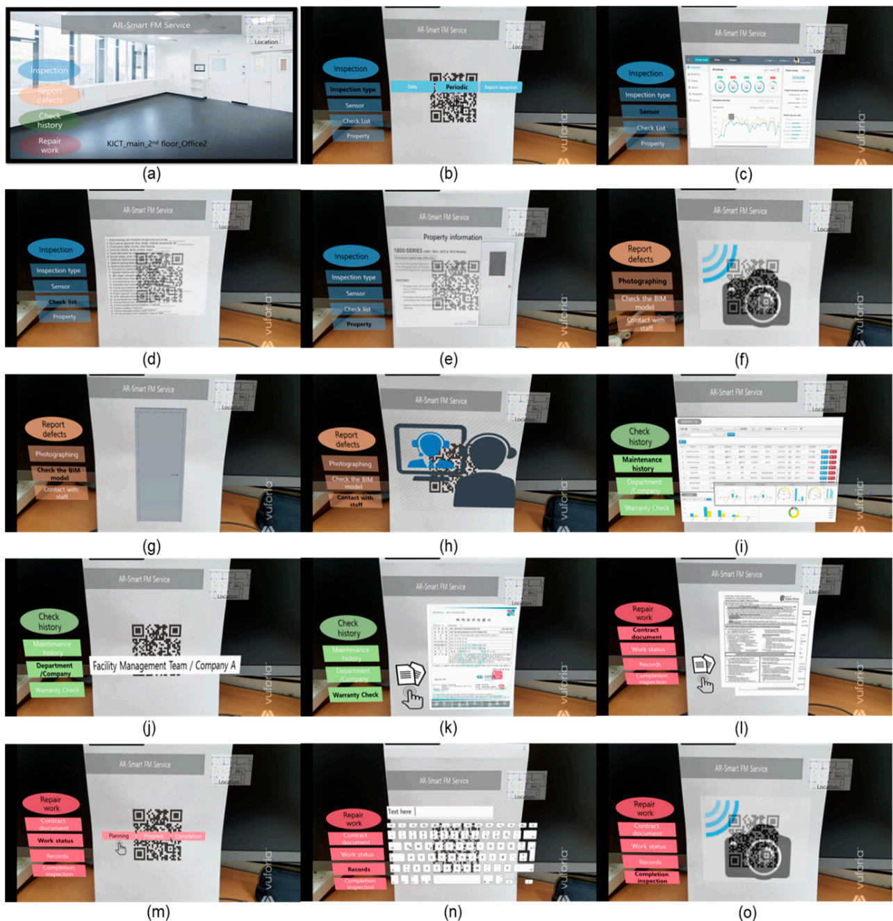
Figure 14. Screenshots of prototype system running the (a) Start menu, (b) Inspection-Inspection type, (c) Inspection-Sensor, (d) Inspection-Check List, (e) Inspection-Property, (f) Report defects-Photographing, (g) Report defects-Check the BIM model, (h) Report defects-Contact with staff, (i) Check history-Maintenance history, (j) Check history-Department/Company, (k) Check history-Warranty Check, (l) Repair work-Contract document, (m) Repair work-Work status, (n) Repair work-Records and (o) Repair work-Completion inspection.
