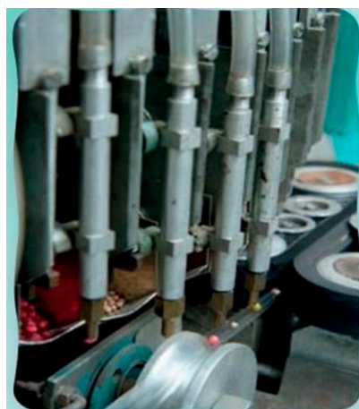
Figure 5. Air suction seed metering device ( https://www.sedos.sk/Data/1049/UserFiles/SEDOS%20Catalogue%202012%20ENG.pdf (accessed on 8 October 2021)).
