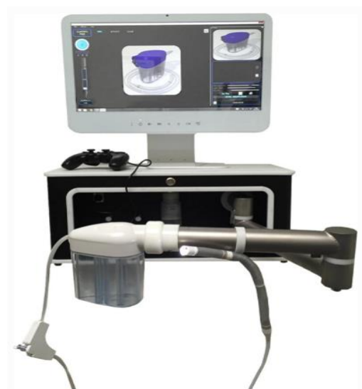
Figure 8. Endotics (ERA Endoscopy SRL, Cascina, Italy) (with permission from Endotics, http://www.endotics.com/ , 29 November 2021). The Endotics system is composed of a workstation and a hand-held console which drives a steerable probe through the colon lumen.
