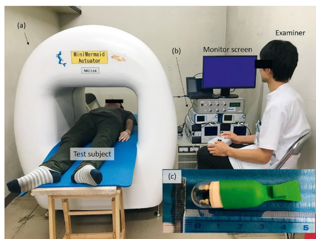
Figure 15. Self-propelling capsule endoscope (Osaka Medical College, Takatsuki, Japan). (a) The patient was examined with the self-propelling capsule endoscope (SPCE) using the New MiniMermaid System. (b) Magnetic field generator. (c) Body of the SPCE [43].
