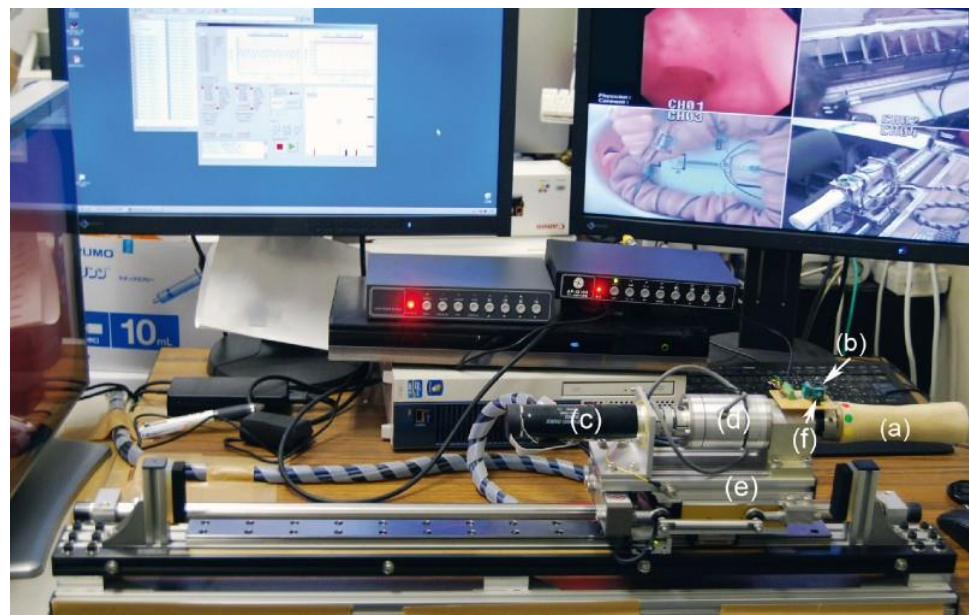
Figure 12. Components of master unit of Endoscopic Operation Robot Ver. 3 (EOR; Kyushu Institute of Technology, Kitakyushu, Japan). (a) Rotating knob, (b) mini joystick, (c) rotary motor, (d) torque sensor, (e) load cell, (f) circuit switch [37].
