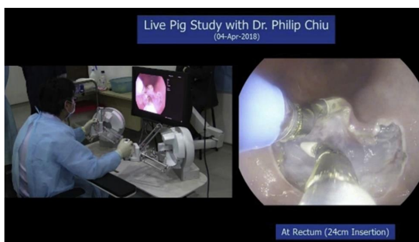
Figure 1. Endomaster EASE System (EndoMASTER Pte, Singapore) [11]. Colonic endoscopic submucosal dissection performed using the latest version of the EndoMaster EASE System. Robotic ESD was performed by grasping the mucosa with the robotic grasper and dissecting the submucosal plane using the needle-type dissecting knife with electrocautery.
