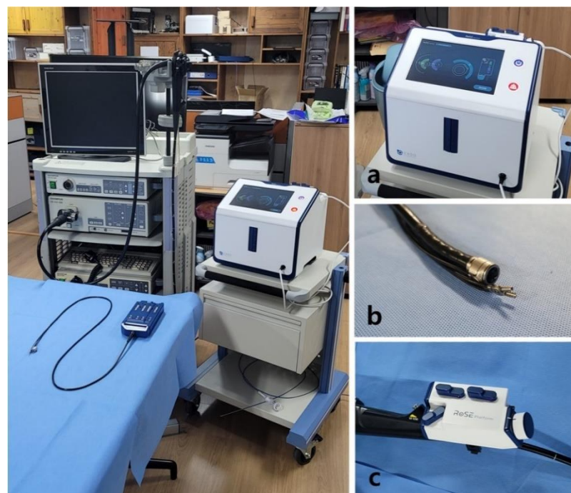
Figure 5. ROSE (Endorobotics, Seoul, Korea) (with permission from Endorobotics, Seoul, Korea). (a) Actuation station. (b) Robotic manipulator attached to the distal end of the conventional endoscope. (c) Intuitive user interface.
