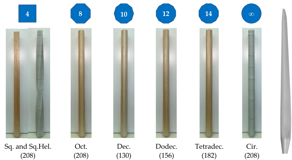
Figure 1. Polygonal cross-sectional towers and blade (LM-Glasfiber) used in the present study (the numbers in parentheses are the number of pressure taps on the towers).
