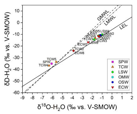
**Figure 6.**  $\delta$ D-H<sub>2</sub>O vs.  $\delta$ <sup>18</sup>O-H<sub>2</sub>O (in‰ vs. V-SMOW) binary diagram for water samples collected from Massaciuccoli Lake. Symbols as in Figure 1b. Global meteoric water line (GMWL:  $\delta D = 8 \times \delta^{18}O + 10$  [88]), local meteoric water line (LMWL:  $\delta D = 7.6 \times \delta^{18}O + 7.5$  [47]) and local evaporation line (LEL:  $\delta D = 5.4 \times \delta^{18}O - 5.9$  [47]).
