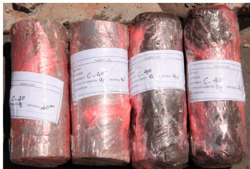
Figure 2. Undisturbed samples.
