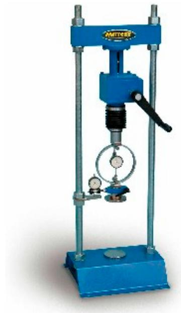
Figure 3. Unconfined compression test equipment.
