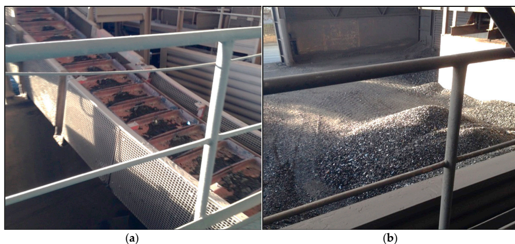
Figure 1. (a) Transport and cooling of cupola slag in trays; (b) detail of the stockpile at the plant.
