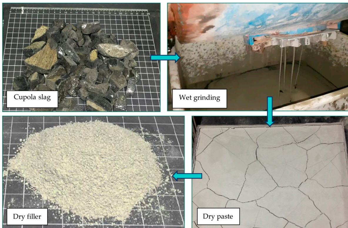
Figure 2. Scheme of the recovery process of cupola slag.
