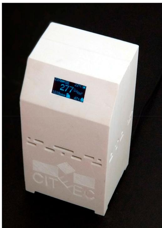
**Figure 3.** The air quality monitoring devices.
