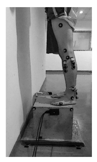
**Figure 1.** The experimental setting comprising the electromyographic (EMG) recording electrodes, marker set, and force plate used for motion analysis.
