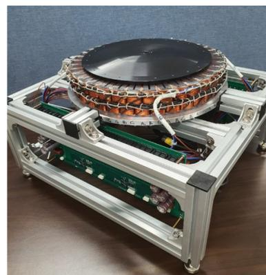
(a) Top of the test maglev system (b) Side of the test maglev system
