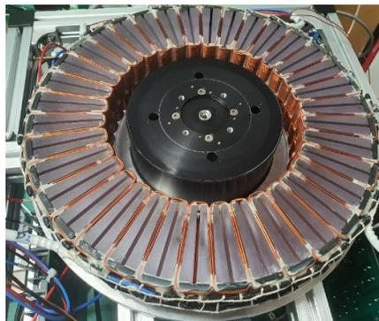
(a) Stator and sensor base of maglev system
