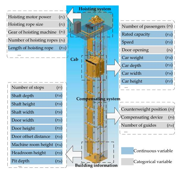
Figure 2. Functional requirements of a customized elevator.
