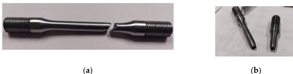
Figure 3. (a) Image of AISI 4145 smooth specimen tested in H_2 ; (b) Image of AISI 4145 smooth specimen tested in N_2 .
