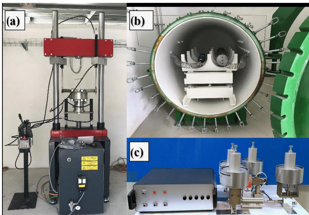
Figure 2. \Delta H Lab test: (a) Servo-hydraulic machine for small scale tests, (b) Inert security chamber for full scale tests, and (c) High-Pressure-Concentration-temperature (HPCT) for adsorption tests.
