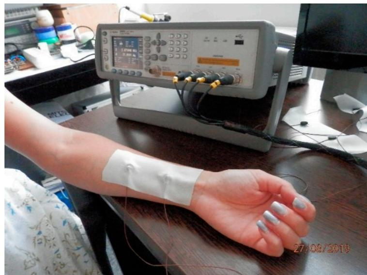
**Figure 13.** The used test bench image for total bioimpedance measurements and dry polarizable bioimpedance sensor location on the arm of the subject.
