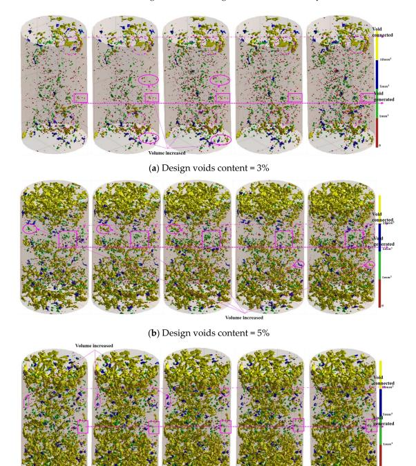
of 7% increased from 6.61% to 8.31%. This reveals that the sample with higher design void content has a higher risk of damage under freeze–thaw cycles.
