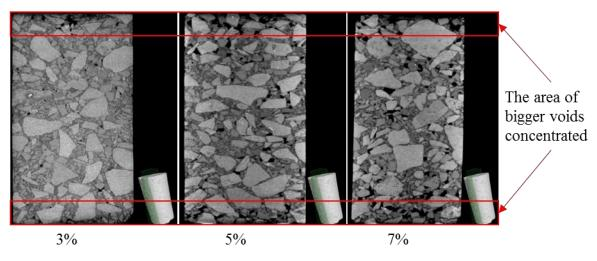
Figure 5. Air void distribution of different samples' determined from 2D slices (vertical direction).
