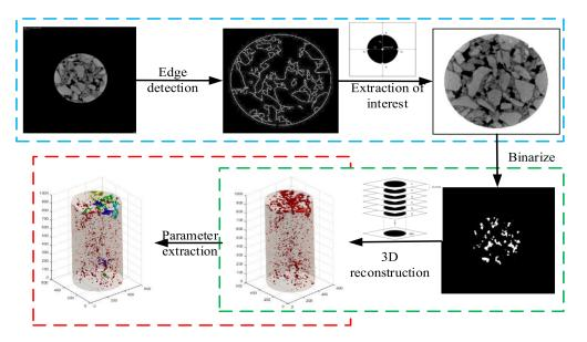
Figure 3. Imaging processing technique [24].
