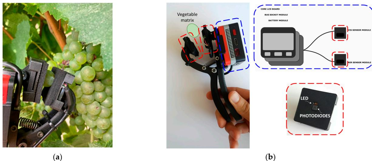
**Figure 1.** (a) Prototype clamp wrapping the sample; (b) prototype layout.
