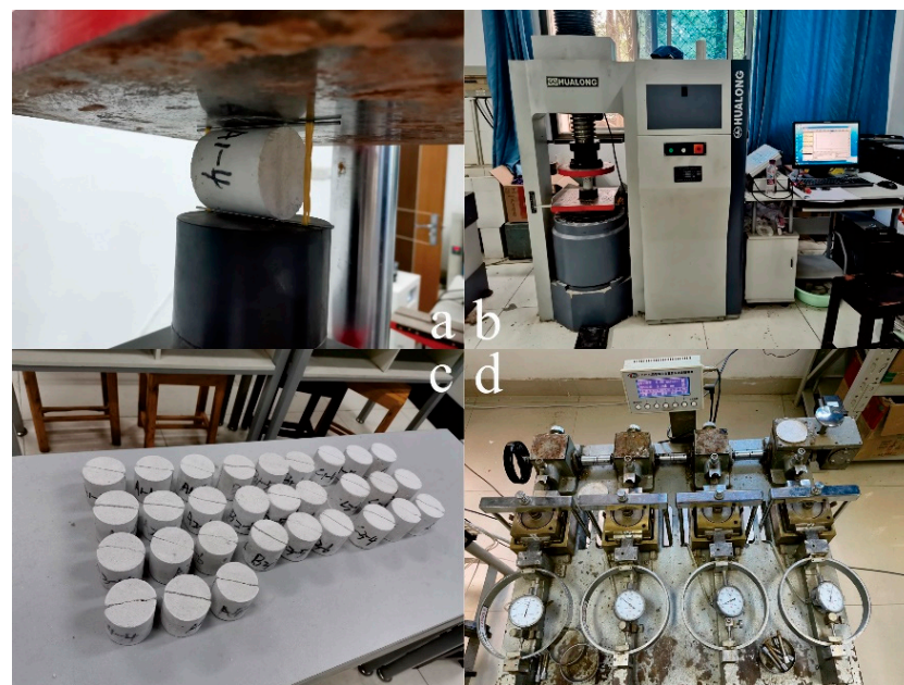
Figure 5. (a) Splitting tensile strength test, (b) uniaxial compression test, (c) specimen, (d) direct shear test.
