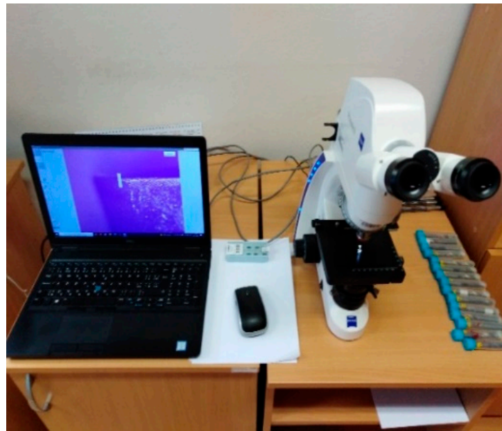
Figure 8. Measurement and analysis of flank wear on the cutting insert by Carl Zeiss Primotech D/A ESD microscope.
