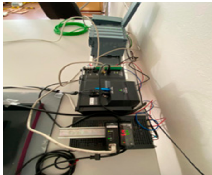
Figure 3. Measuring scheme of LTS, containing amplifier IL-1000, profinet module DL-PN1, PLC module Siemens 1511C.
