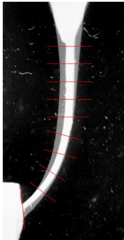
**Figure 2.** Illustration of the measurement points, measured every 1 mm, perpendicular to the axis of the duct.
