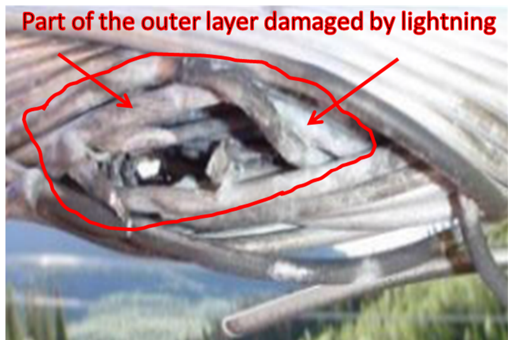
Figure 8. Image of conductor outer layer damaged by lightning [39].
