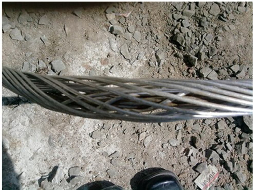
Figure 9. Bird caging in transmission conductor [90].
