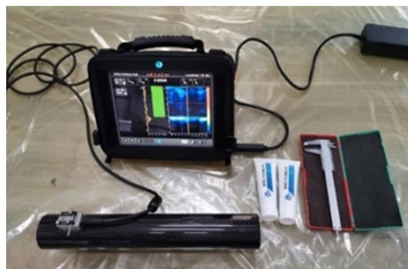
**Figure 14.** Field diagram of CFRP shaft tube ultrasonic scanning experiment.
