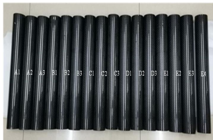
Figure 11. Specimen of CFRP shaft tube.
