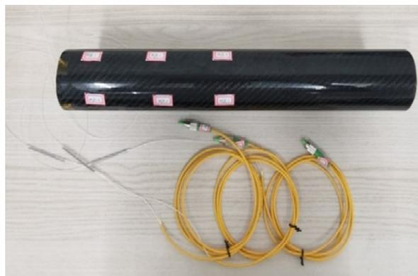
Figure 17. CFRP shaft tube pasted with FBG sensor.
