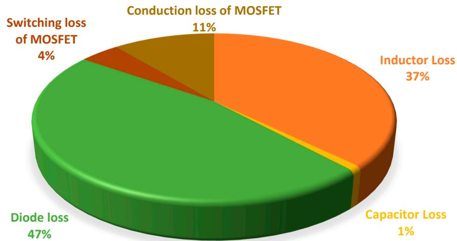
Figure 10. Converter loss breakdown chart for HG-SIQBC topology.
