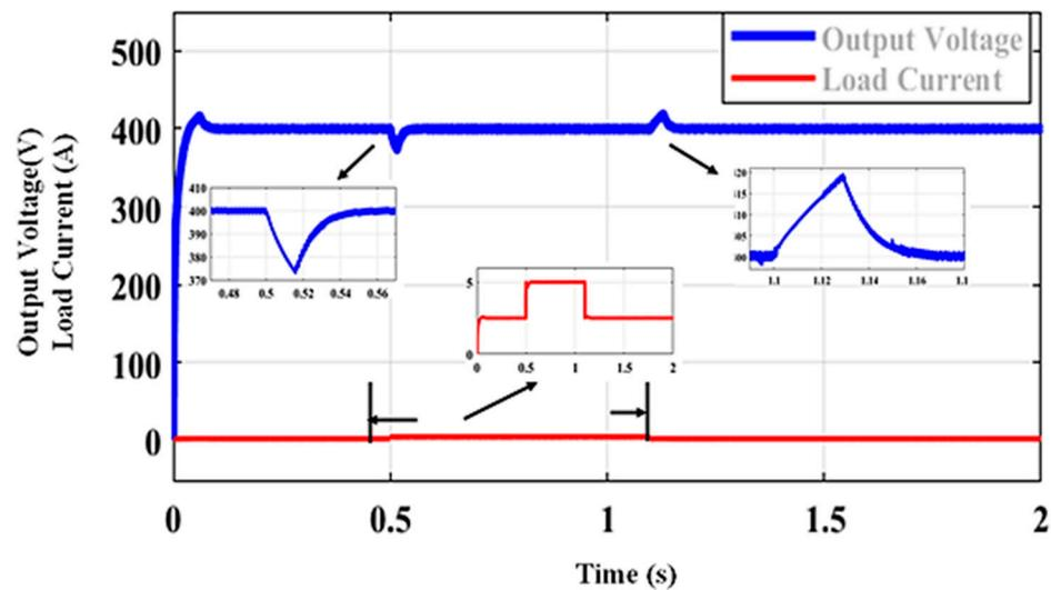
Figure 12. HG-SIQBC-output voltage and current when subjected to a load change for  $V_{in} = 75$  V.
