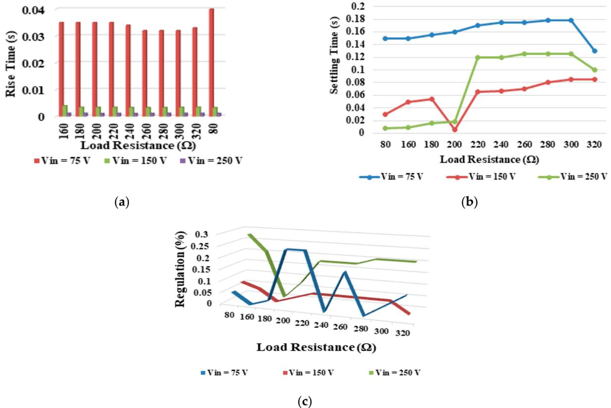
Figure 15. Performance analysis of HG-SIQBC: (a) rise time; (b) settling time; (c) regulation.
