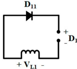
Figure 9. HG-SIQBC—equivalent circuit to find the voltage stress across diode  $D_1$ .
