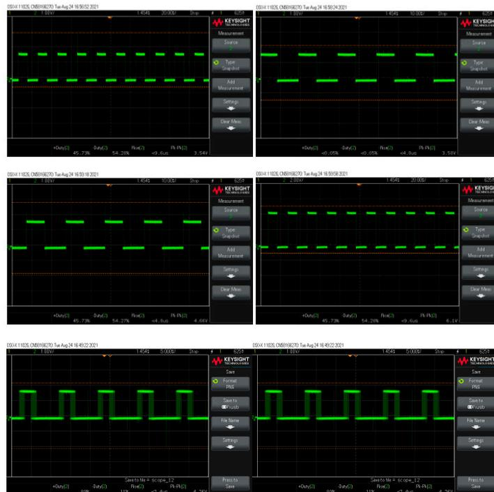
Figure 21. Gate pulses for switches  $S_1$ – $S_6$ .
