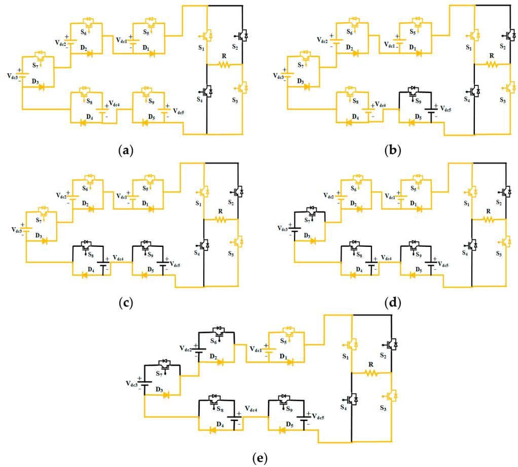
Figure 17. (a–e) Equivalent circuit for different modes during positive cycle of output voltage.
