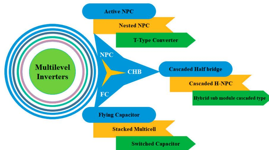
**Figure 1.** Multilevel inverter classifications.
