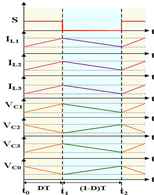
Figure 4. Theoretical waveforms of the proposed HG-SIQBC. (Ton and Toff are differentiated with dotted lines with pink and blue backgrounds respectively).
