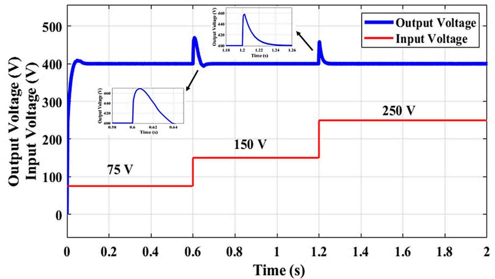
Figure 13. Output voltage response with input voltage variation for proposed HG-SIQBC.
