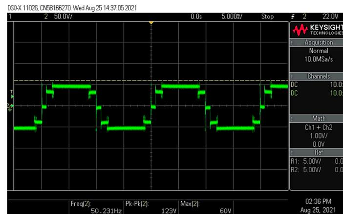
Figure 22. Output voltage waveform (five levels).
