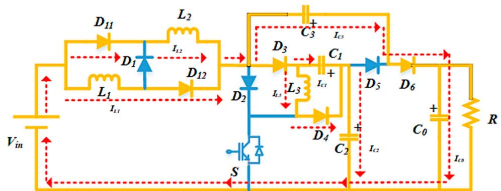
Figure 6. HG-SIQC—equivalent circuit for Mode II. (The conducting portion of the circuit is shown in Yellow color with the current flow in dotted lines).
