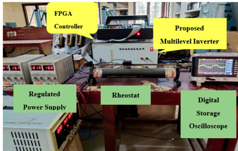
Figure 20. Hardware setup for proposed multilevel inverter.
