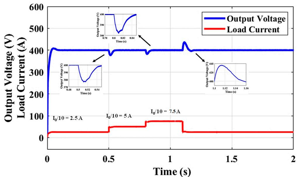
Figure 14. Output voltage response with step change in load resistance for proposed HG-SIQBC for  $V_{in} = 75$  V.
