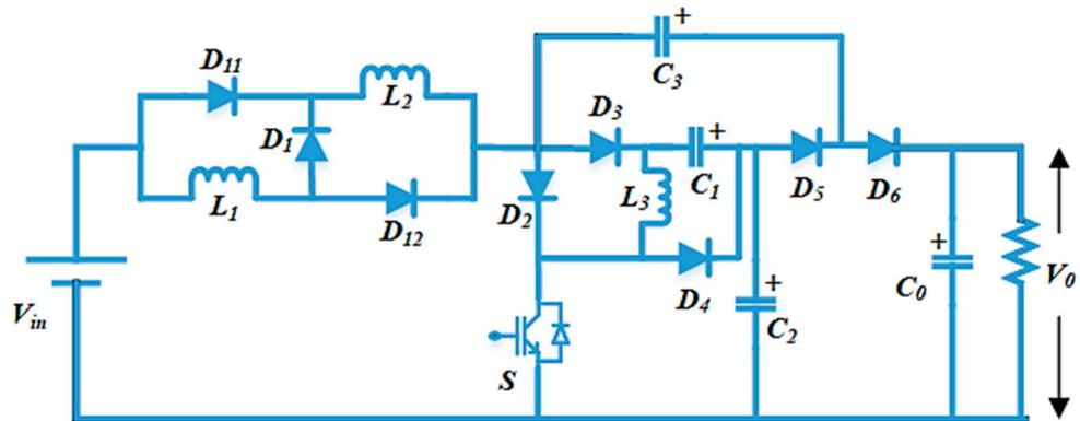
Figure 3. Circuit diagram of proposed HG-SIQBC.
