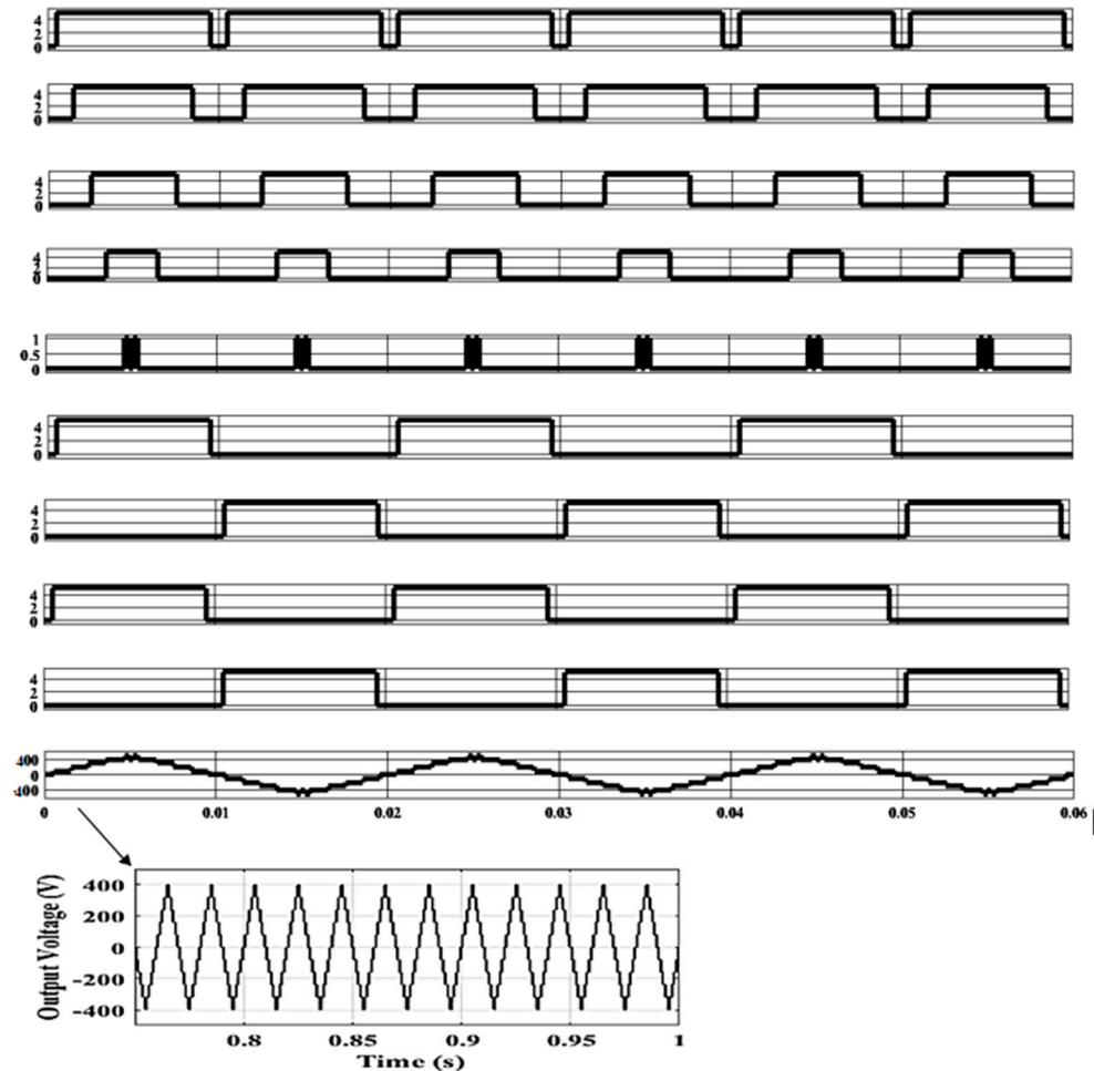
Figure 19. Pulse waveforms and output voltage waveform of the proposed inverter.
