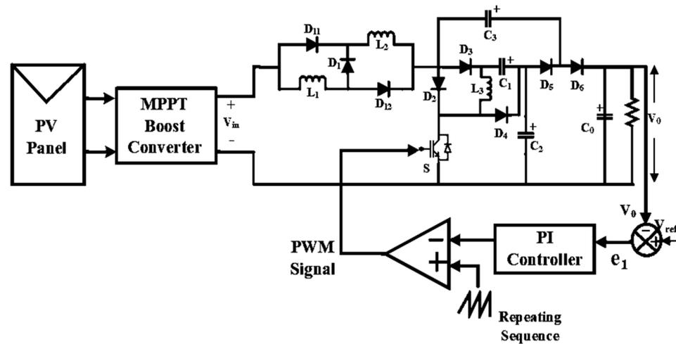
Figure 11. Block diagram of closed-loop control for proposed HG-SIQBC.
