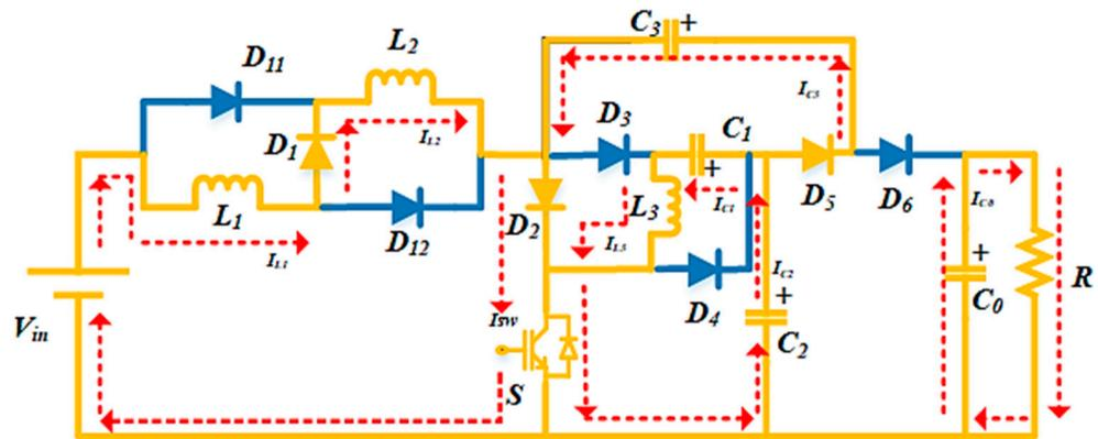
Figure 5. HG-SIQBC—equivalent circuit for Mode I. (The conducting portion of the circuit is shown in Yellow color with the current flow in dotted lines).
