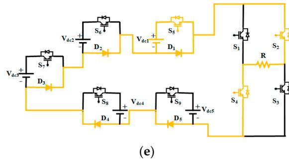
Figure 18. (a–e) Equivalent circuit for different modes during negative cycle of output voltage.
