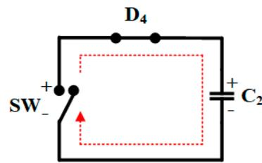
Figure 8. HG-SIQBC—equivalent circuit to find the voltage stress across the switch. (The current flow is given in dotted lines).
