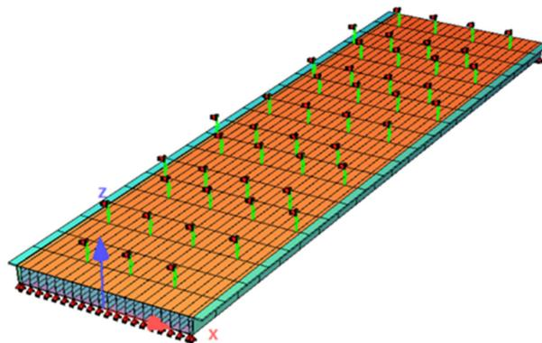
**Figure 3.** Numerical model of web-core sandwich panel FRP bridge in Puurs with SDOF pedestrians.
