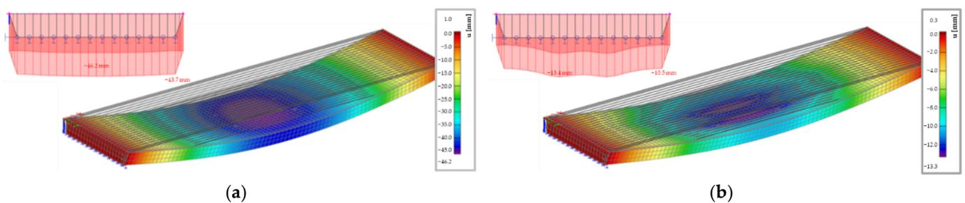
**Figure 2.** Longitudinal and transverse deflection under (a) a uniformly distributed load (LC3) and (b) a service vehicle (LC4).
