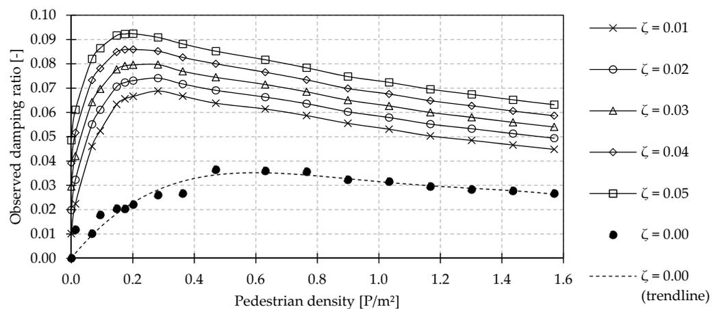
**Figure 4.** Calculated damping ratio as a function of pedestrian density.
