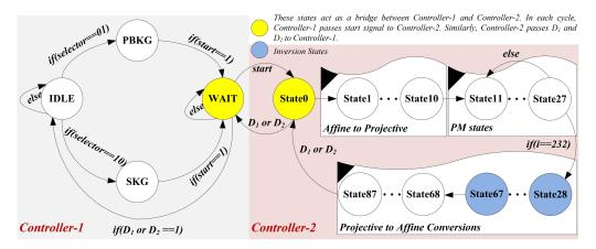
Figure 4. FSM controller of our proposed ECDH accelerator architecture.
