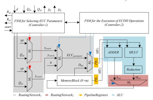
Figure 3. Proposed ECDH accelerator architecture for key-agreement.
