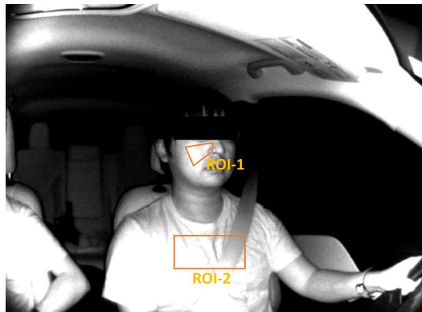
**Figure 2.** Position of both ROI-1 and ROI-2 as seen by the ToF camera. The grayscale intensity and depth information from ROI-1 are used for HR measurement, and the depth information from ROI-2 is used for RR measurements.
