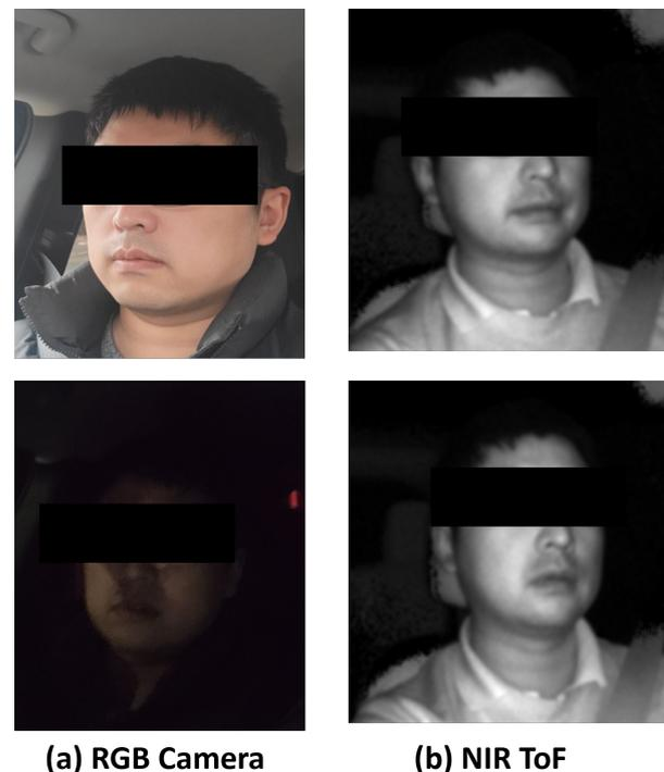
**Figure 6.** The user's face seen by an RGB camera (a) in both bright (top) and dark (bottom) conditions versus the user's face seen by the ToF camera in both bright (top) and dark (bottom) conditions.
