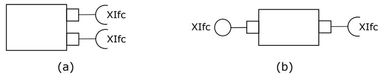
**Figure 15.** Cases searched in real-life projects: (a) Case 1: a class having more than one port that requires the same interface. (b) Case 2: a class that provides and requires the same interface at multiple ports.
