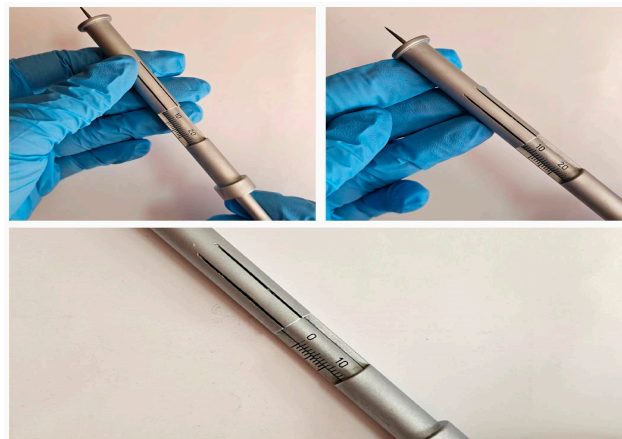
Figure 1. Skin thickness measuring instrument length 0–30 mm.
