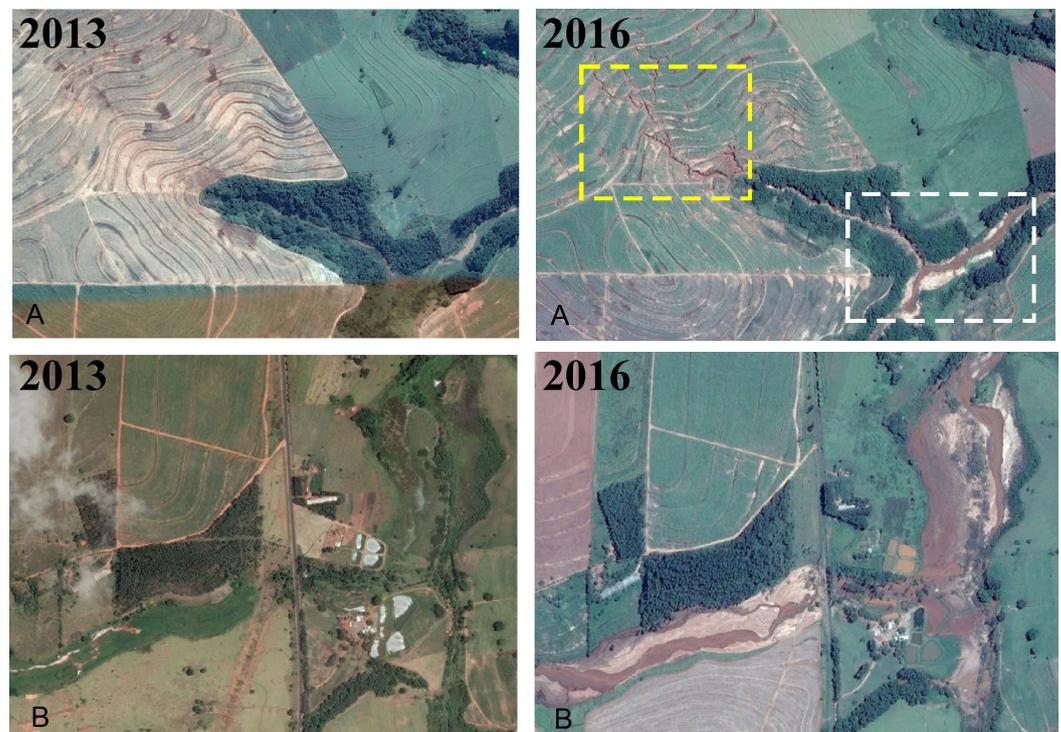
**Figure 7.** Aerial view of pre and post EN 15–16 landscape in a rural area of Nossa Senhora das Graças, Paraná state, Brazil: (A) at the upstream sector, extensive and deep linear erosional features (gullies) were developed on a sugarcane plantation (yellow square) as well as deposition of sediments generated on the slopes (white square); (B) at the downstream sector of the same basin, the depositional processes were predominant. Source: Google Earth.
