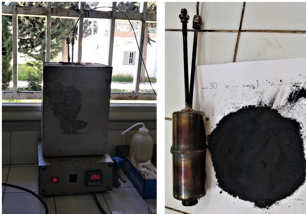
**Figure 1.** Reactor and furnace used to produce activated carbon.
