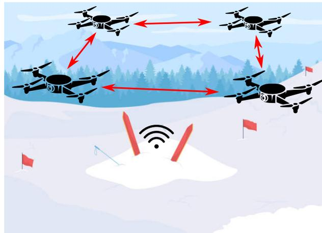
**Figure 15.** Simulation Test #5—Representative example of a SAR activity for a missing skier equipped with ARTVA device. The red arrows indicate the communication link between the UAVs.
