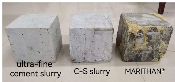
**Figure 4.** Grouting specimens with different grouting materials.
