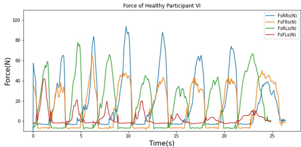
**Figure 4.** Force sensor reading. Force sensor on rear right side (FsRRs (N)), force sensor on rear left side (FsRLs (N)), force sensor on front right side (FsFRs (N)), and force sensor on front left side (FsFLs (N)).
