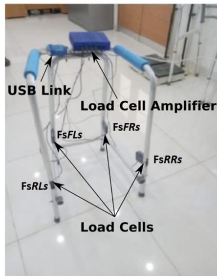
Figure 1. Smart Walker with on board sensors.
