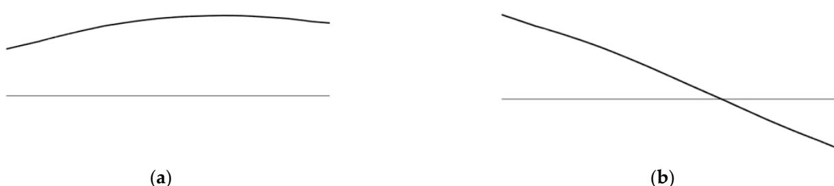
**Figure 3.** Mode shapes of the first two critical speeds: (a) mode shape for critical speed 1588 rad/s; (b) mode shape for critical speed 3276 rad/s.
