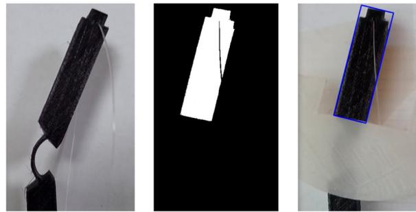
**Figure 8.** Object detection using image processing. (left) Original image of the 3D-printed finger. (middle) Segmented object region represented with white pixels in the segmented binary image. (right) Detected object bounded with an extracted minimal rectangle (blue-colored rectangle).
