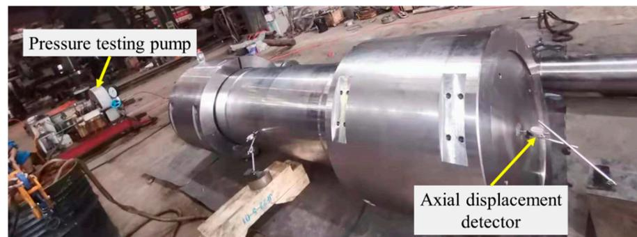
Figure 10. Pressure system for testing the rock cabin.
